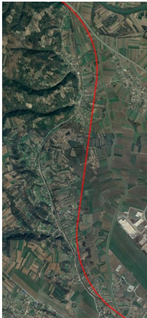
**Figure 42. Deviation of the new railway (red line) in reference to the existing one (black one)**
