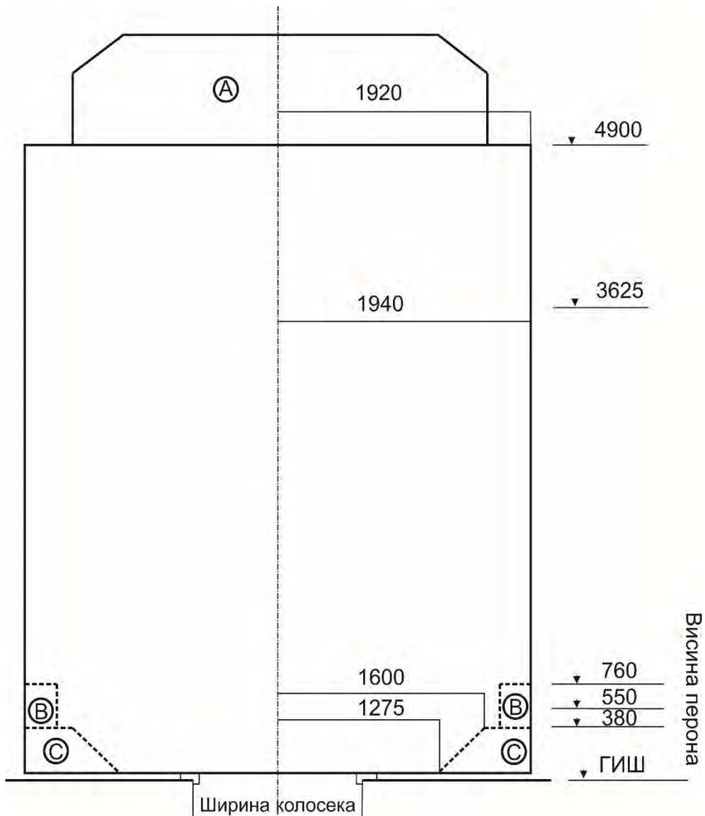
A – Pantograph movement space
