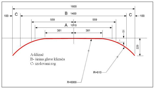
Figure No 1. – Dimensions of pantograph
