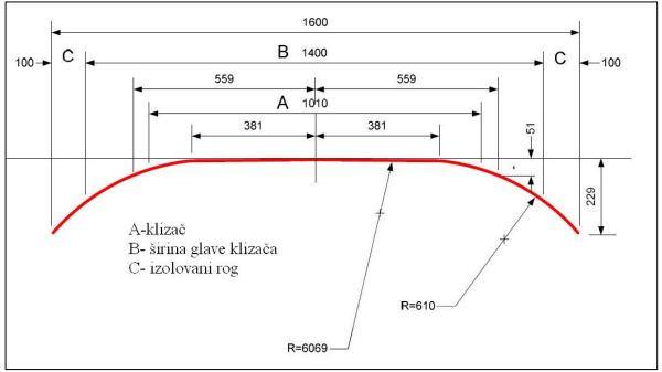
Figure No 1. – Dimensions of pantograph
