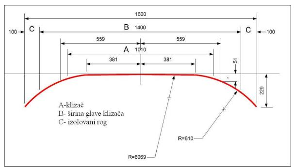
Figure No 1. – Dimensions of pantograph
